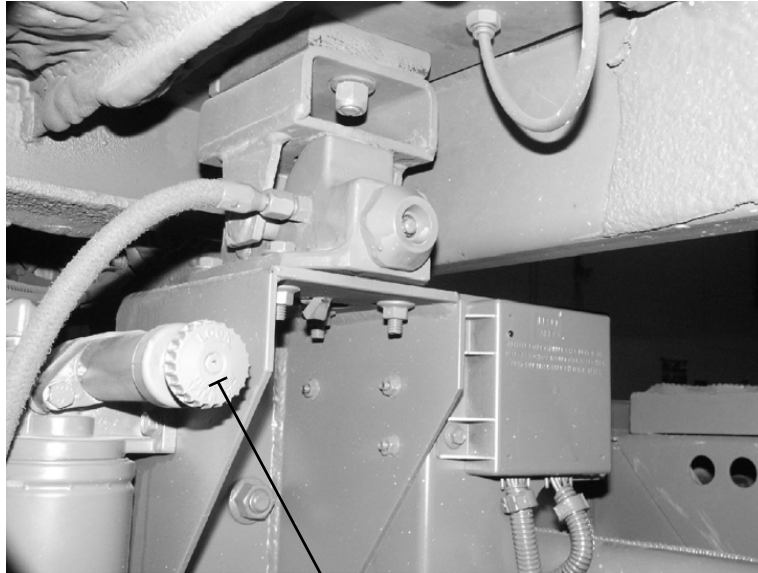
FUEL PRIMING PUMP PLUNGER (LEFT SIDE OF TRUCK)
