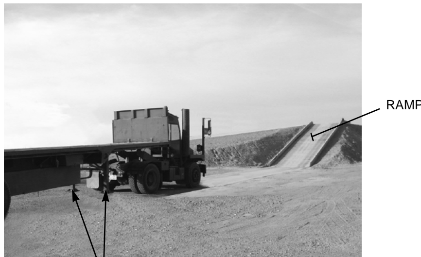
LANDING GEAR HAS 6-8 IN (15-20 CM) CLEARANCE
